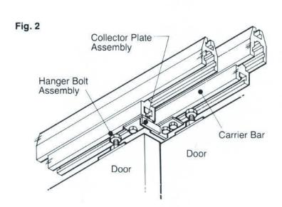
Shown on this page is a Parallel Door System using the Alloy Light "Fitzroy" Door Track.
